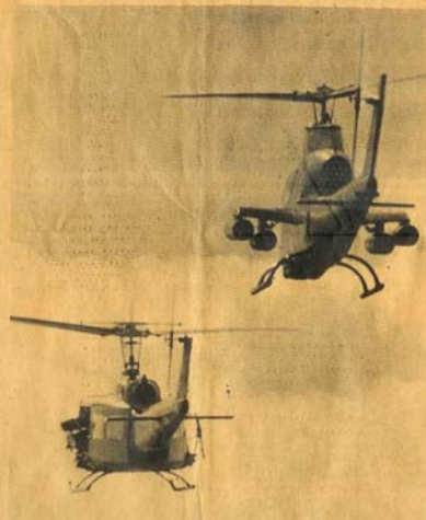
READY TO TACKLE ENEMY -- Armed with two mini-guns, a 40mm grenade launcher, machine gun and 76 rockets, the Nighthawk team of Huey (left) and Cobra helicopters are ready to tackle the enemy during night missions for the 1st Air Cavalry Division.
